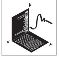
For timing measurements, the Modulation Domain's view of time interval vs. time allows you to both see and quantify timing jitter directly—taking you one step beyond the Time Domain's qualitative view.
